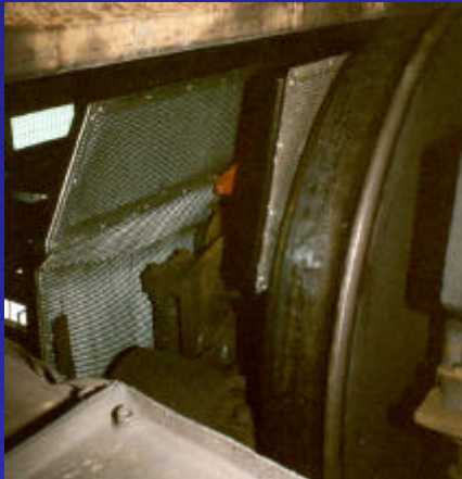
Wheel with surface irregularities
