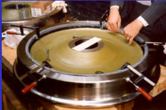
Application of dampers on a well smoothed wheel
